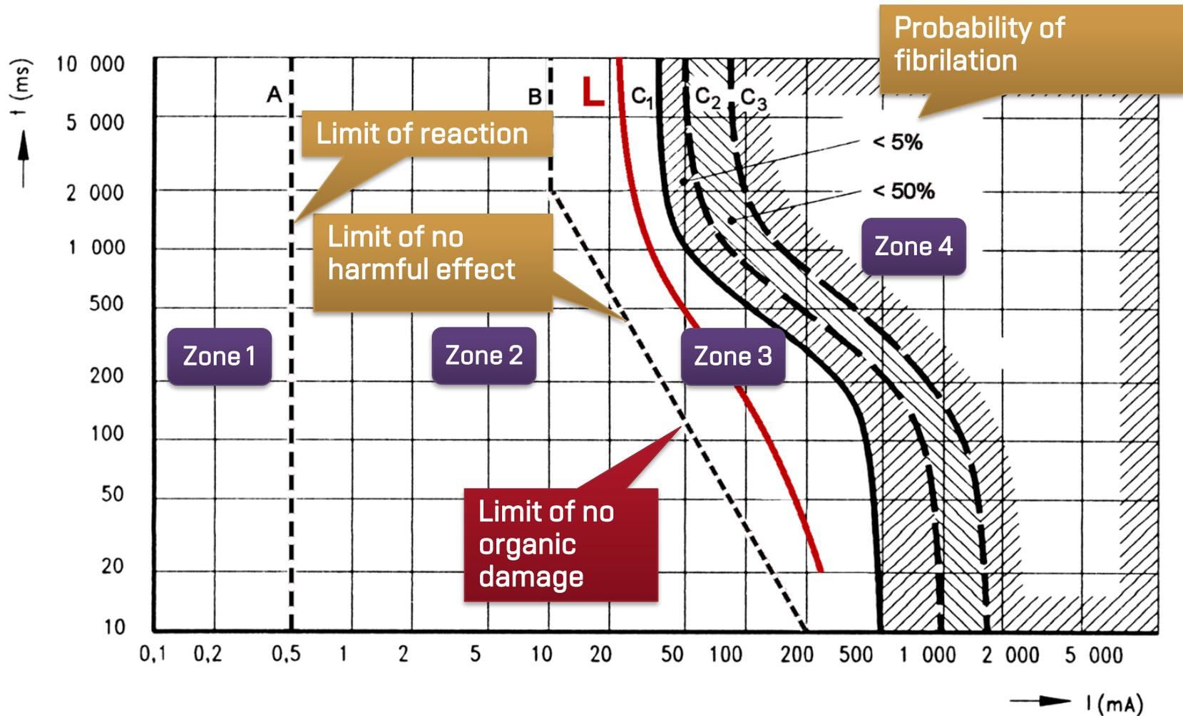
This diagram is valid for AC 15-100 Hz , way of current left hand to both legs
