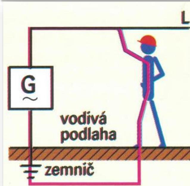
Indirect contact with exposed conductive part
